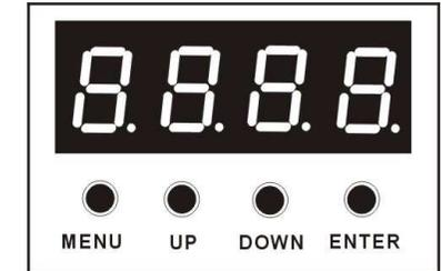
Normally, the LED will display current DMX address code, as like: “DMX Address: 001”. Press<MENU> to enter the main menu; press <UP> or <DOWN> to scroll in the menu or submenu options; Press <ENTER> to confirm your selection. Any time press and hold <UP> or <DOWN>,the value will rapidly change and stop when released. Once the value is set, press <ENTER> again to save and exit to the main menu.
